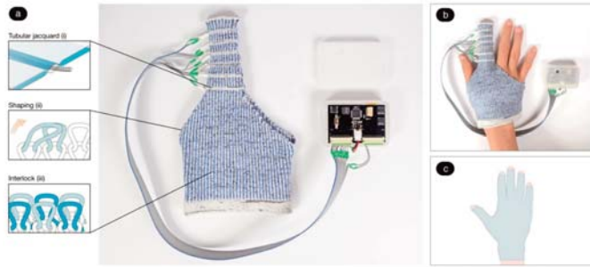
(a) KnitDema system in which the finger sleeve is knitted with a combination of (i) tubular jacquard, (ii) shaping and (iii) interlock structure. The tubular structure creates “channels” to incorporate shape-memory alloy springs. The substrate also uses a shaping structure to conform the substrate to the rest of the fingers. (b) KnitDema finger sleeve device worn on a hand. (c) Future implementation of a full-hand KnitDema device. Image: Hybrid Body Lab, Cornell University
